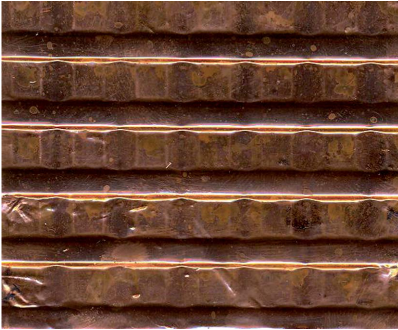
Fig. 6.4 Copper-faced bitumen roofing sheet
