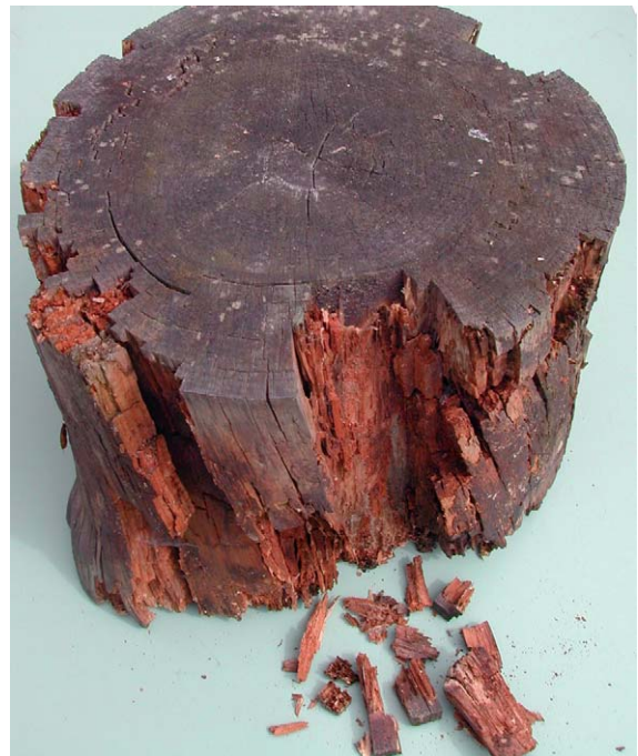
Fig. 4.18 Deterioration of sapwood timber illustrating the relative durability of heartwood over sapwood
