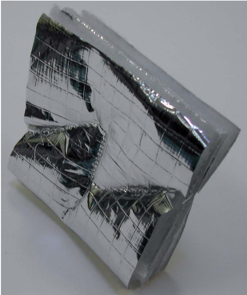
Fig. 13.3 Multi-layer aluminium foil insulation system
